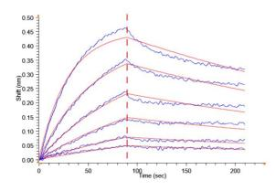
Loaded Human HGF R, hFc Tag on ProA-Biosensor can bind Human HGF, His Tag with an affinity constant of 4.32 nM as determined in BLI assay (Gator® Prime).
